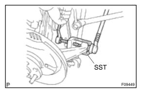
(b) Using SST, disconnect the No. 2 lower suspension arm. SST 09610–20012
