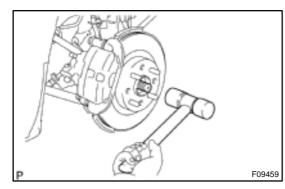
11. **DISCONNECT DRIVE SHAFT FROM AXLE HUB** Using a plastic hammer, disconnect the drive shaft from the axle hub.
