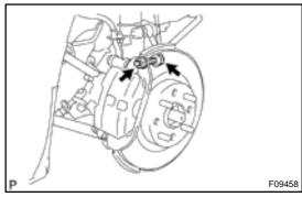
10. REMOVE ONLY VERY BOTTOM BOLT, NUT AND 2 WASHERS OF SHOCK ABSORBER
